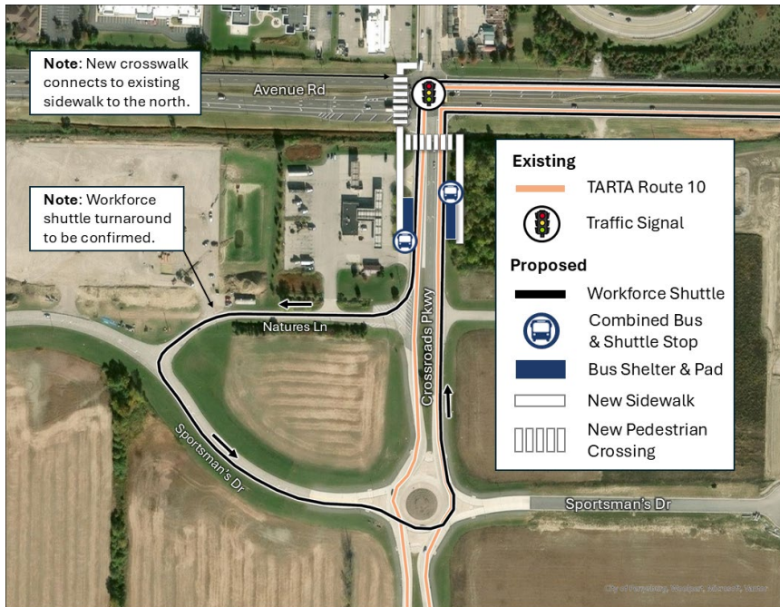
FIGURE 43 – EXAMPLE CONNECTION POINT AT 795 AT CROSSROADS PARKWAY
